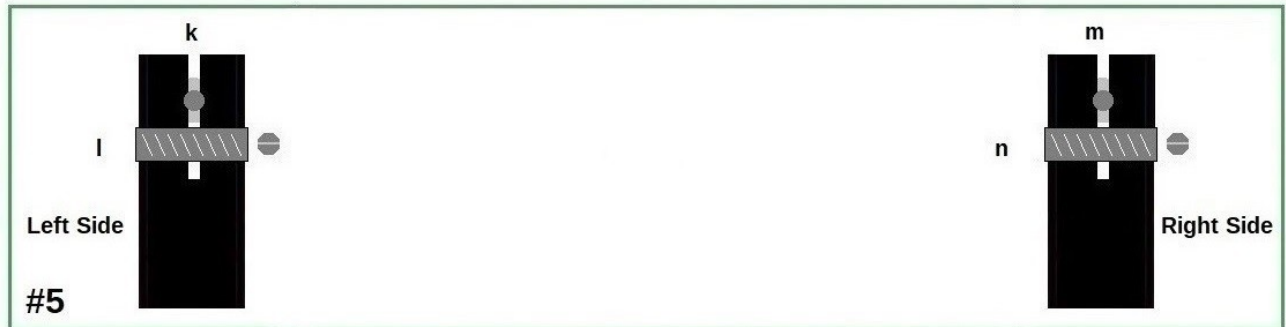
#5k,m Electromagnets' 3" Supports (2, 1" PVC * 3" L w Slots) Side Views #5l,n Hose Clamps (2, 1")
